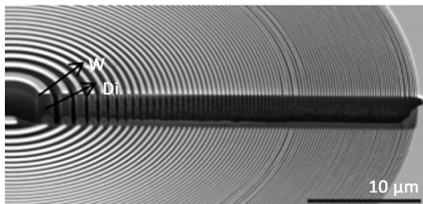
Figure 8. SEM image of W-Di FZP [38]
