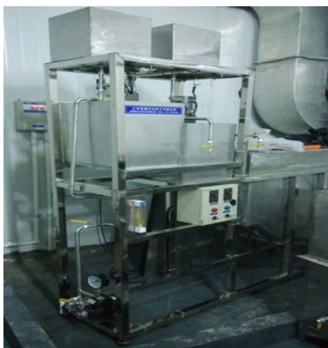
Figure 2. Chemical flocculation precipitation technology experiment platform 图 2. 化学絮凝沉淀技术实验台架
