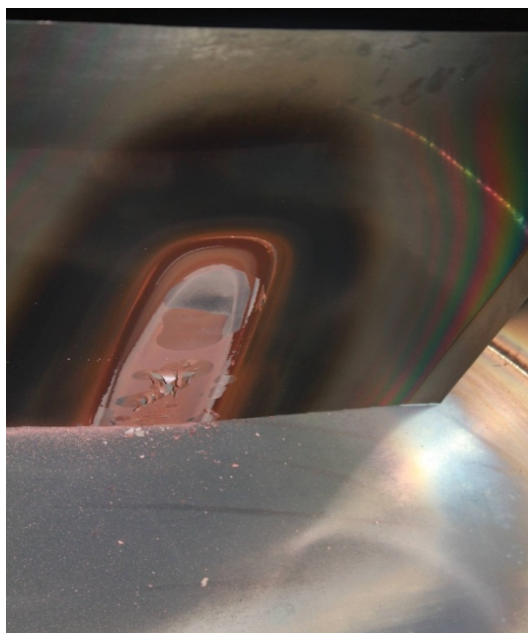
Figure 11. Laser cleaning effect diagram 图 11. 激光清洗效果图
