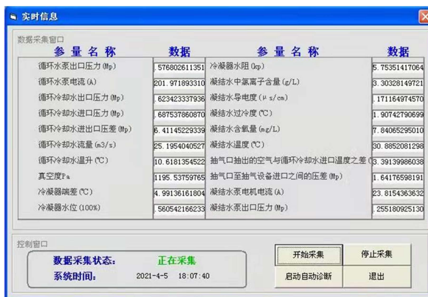
Figure 4. Condenser fault diagnosis system based on BP neural network (acquisition)
