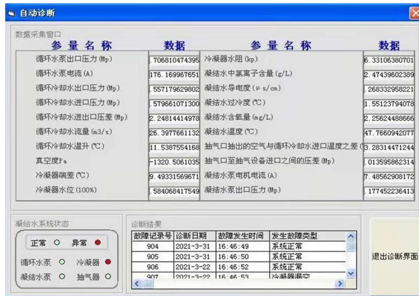
Figure 5. Condenser fault diagnosis system based on BP neural network (diagnosis) 图 5. 基于 BP 神经网络的凝汽器故障诊断系统(诊断)
