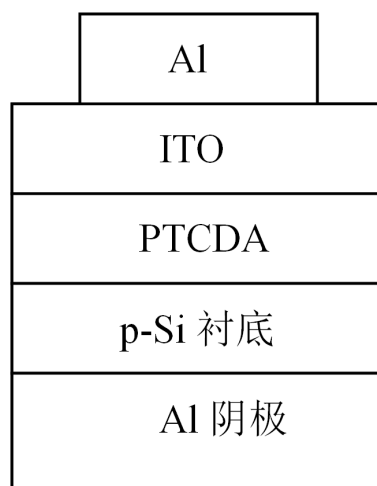
Figure 1. Al/ITO/PTCDA/p-Si/Al barrier device architecture
