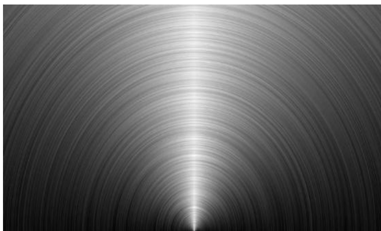
Figure 4. Off axis Fresnel lens for ultra short focal length projection screens 图 4. 用于超短焦距投影屏幕的偏轴菲涅尔透镜
