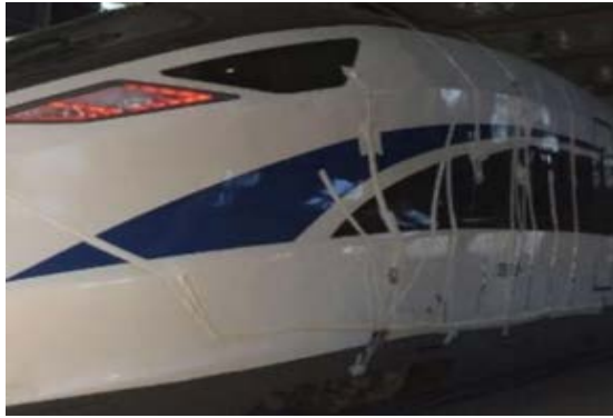
Figure 4. Layout of acoustic excitation measuring points on car body surface 图 4. 车体表面声激励测点布置图
