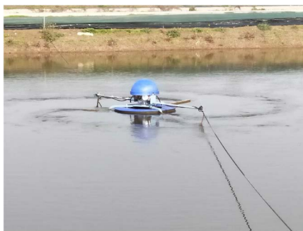
Figure 1. Water agitator and aerator for breeding pool installation 图 1. 育种试验池安装使用的增氧活水机
