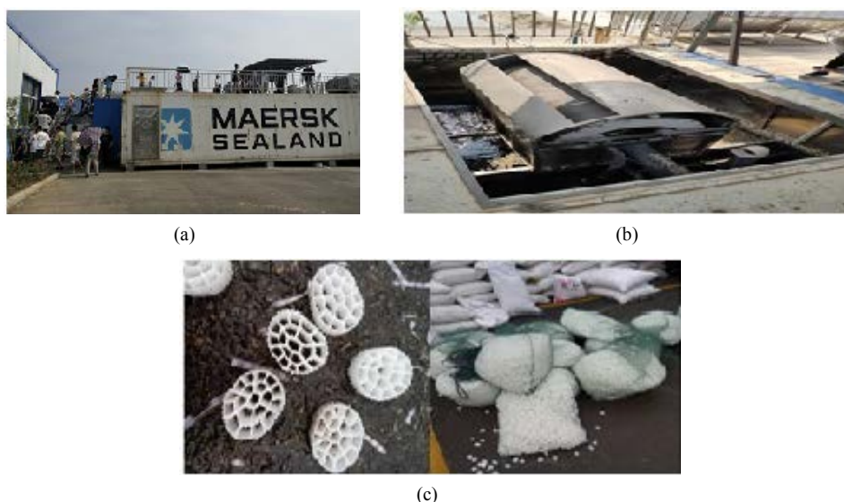
Figure 3. (a) Container recirculating aquaculture system in Dongping, photo taken on May 26, 2019; (b) Integrated water treatment system: integrating filtration, aeration and biofilm treatment; (c) Porous Fluidized Bed Biofilm: The main function of the porous fluidized bed biofilm is to allow microorganisms to multiply rapidly and form biofilm
