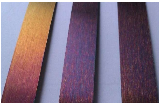
Figure 7. The color of the colored stainless steel when the potential difference is 24 mv 图 7. 电位差为 24 mv 时, 获得的彩色不锈钢的颜色
