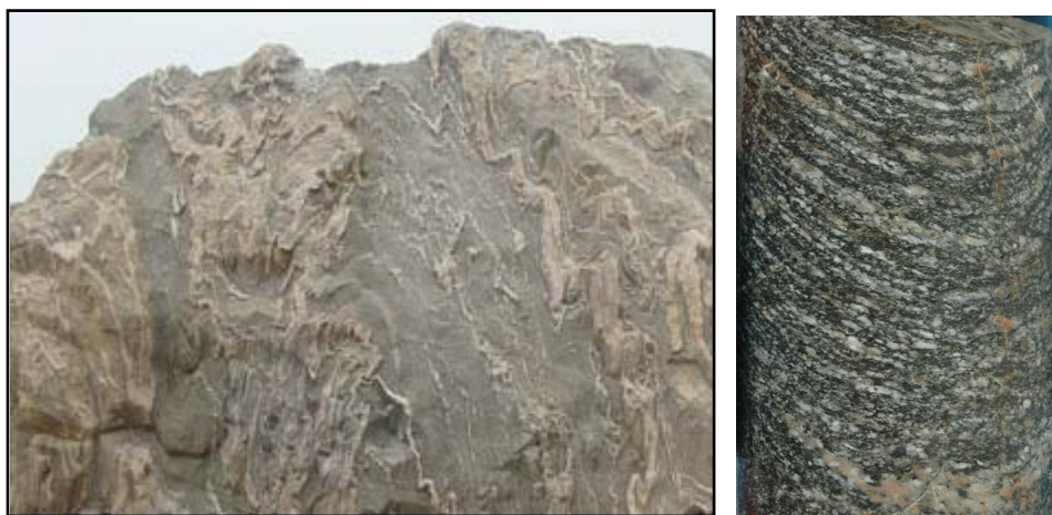
Figure 2. Characteristic of migmatite basal bodies (dark) and vein body (undertone) (left is outcrop, right is core)
