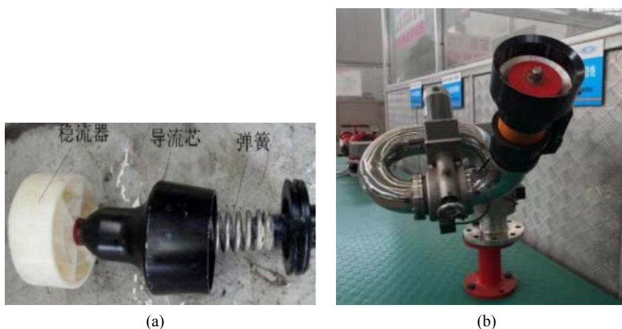
Figure 1. Internal structure of fire sprinkler (a) and site working diagram (b)
