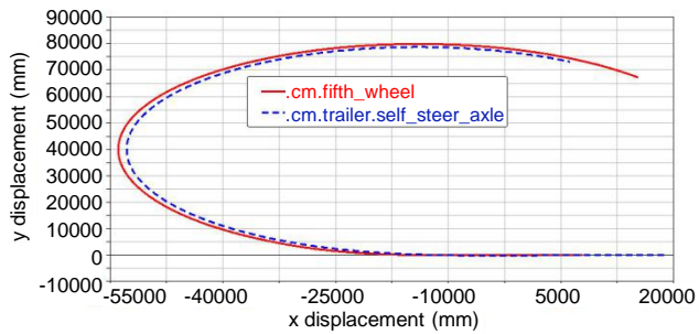
Figure 6. Path-following of self-steering tractor-semitrailer in 360-degree turning test in 360-degree turning test
