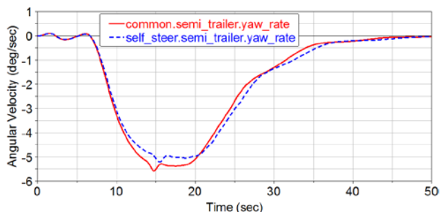
Figure 13. The yaw rate of common and self-steering semi-trailer in 90-degree turning test
