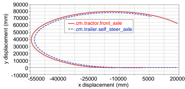
Figure 4. CG trajectory of front axle and trailer third axle of common tractor-semitrailer axle of self-steering tractor-semitrailer
