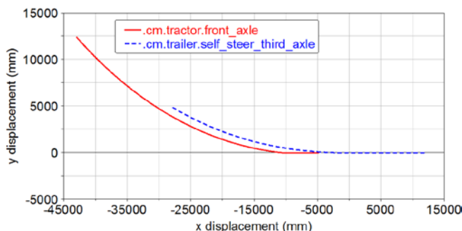
Figure 19. CG trajectory of front axle and trailer third axle of common tractor-semitrailer
