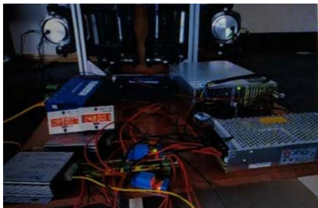
Figure 8. Test bench for electromechanical braking system 图 8. 电机械制动系统试验台
