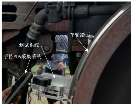
Figure 1. Field test of wheel tread wear 图 1. 车轮踏面磨耗现场测试
