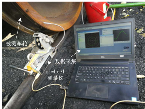
Figure 5. Field test scene of wheel irregularities 图 5. 车轮不圆顺现场测试场景
