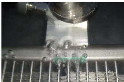
Figure 6. Leakage position after test
