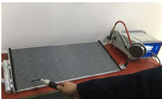
Figure 4. Halogen leak detection 图 4. 卤素检漏
