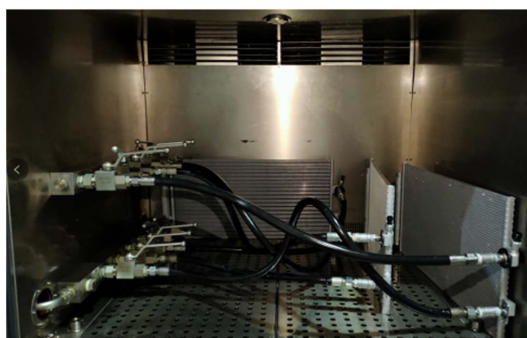
Figure 5. Pressure alternating test
