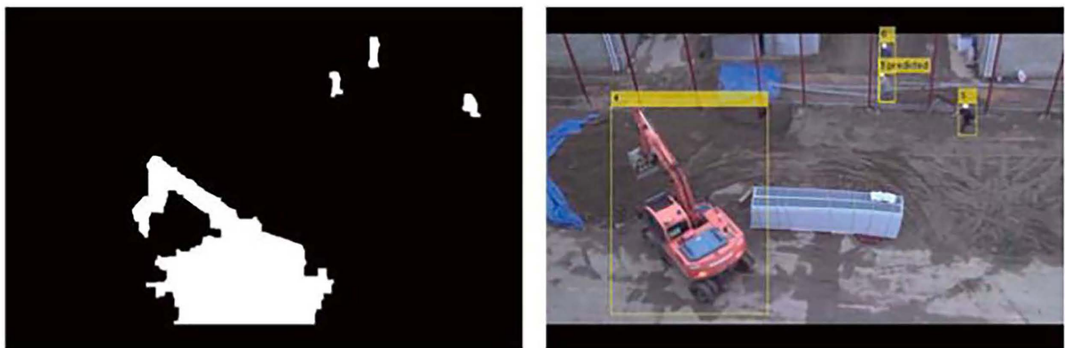
Figure 6. Visual based monitoring of moving object collision accidents 图 6. 基于视觉的移动物体碰撞事故监测
