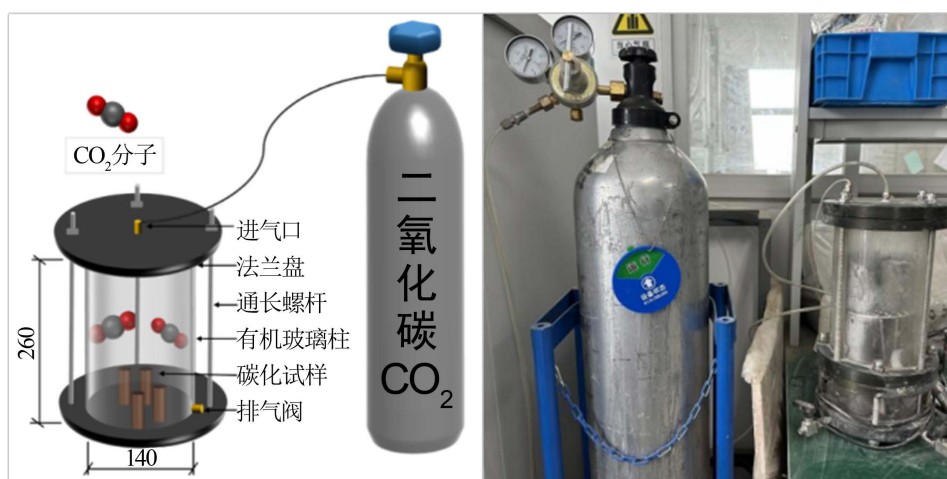
Figure 2. Carbonized reinforcement test device (unit: mm)
