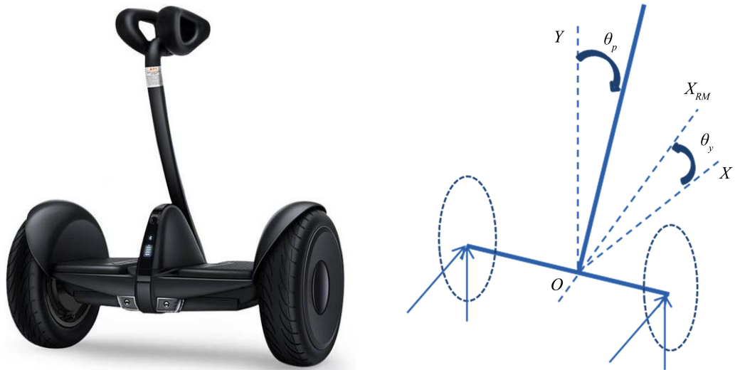
Figure 1. Schematic diagram of the actual two-wheeled balancing vehicle and its coordinate system 图 1. 两轮平衡车实物和坐标系示意图
