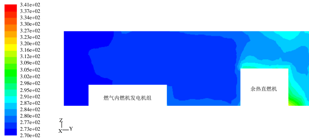
Figure 11. Temperature field in X = 3.95 m 图 11. X = 3.95 m 平面处的温度场
