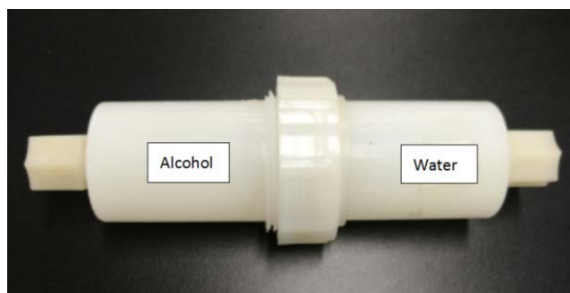
Figure 3. Test device for permeability of ethanol
