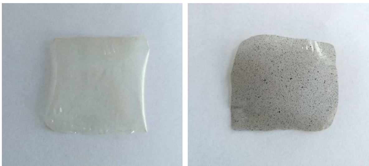
Figure 1. CS membrane (left) and CS-GO membrane (right) 图 1. CS 膜(左)和 CS-GO 膜(右)
