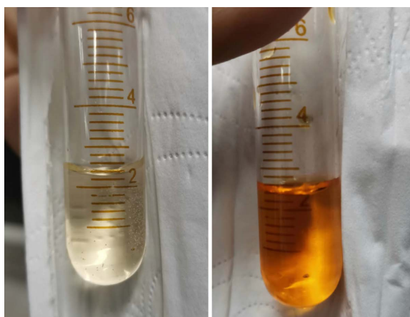
Figure 4. Photocatalytic degradation of alkaline phenol solution in Fenton-like system—left (after degradation); right (before degradation)
