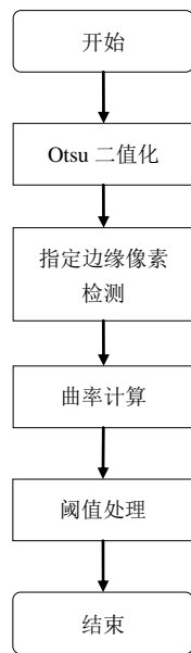
Figure 9. Defects detection flowchart 图 9. 缺陷检测流程图
