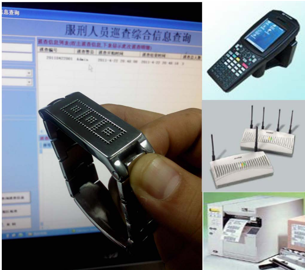
Figure 5. Real figure of RFID tags, collector, wireless AP and bar code printers 图 5. RFID 标签、采集器、无线 AP 和条码打印机实物图
