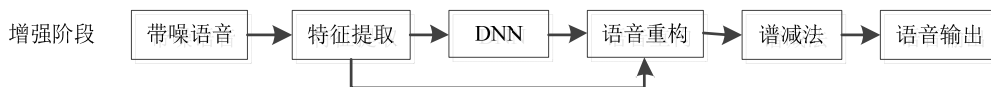
Figure 7. Speech enhancement model based on regressive DNN 图 7. 回归深度神经网络语音增强模型
