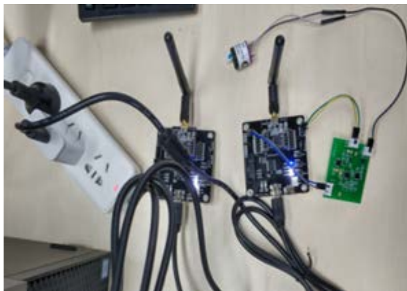
Figure 6. Oxygen concentration collection terminal node
