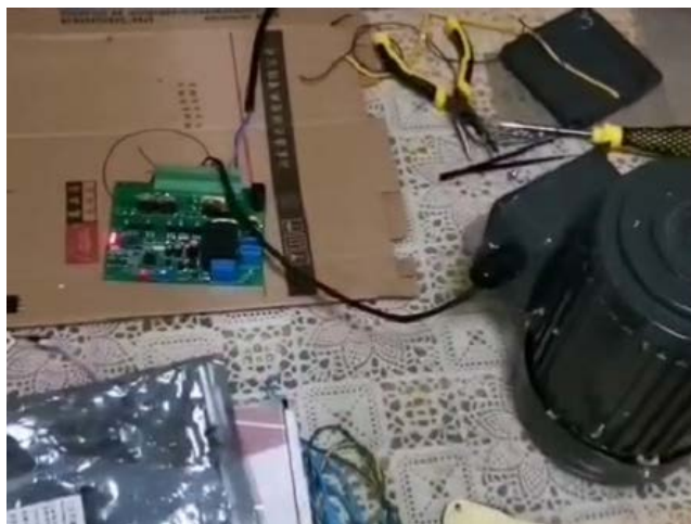
Figure 6. The physical connection picture of cow brush controller 图 6. 控制器实物连接图
