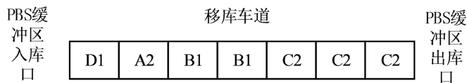
Figure 8. Vehicle information on transfer lane after outbound 图 8. 出库后移库车道车辆信息
