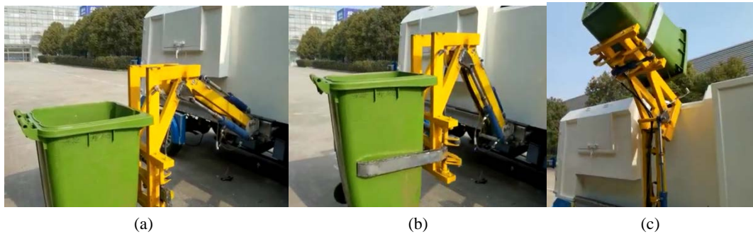
Figure 7. Precise control of garbage bin: (a) forward extension, (b) clamping, (c) lifting 图 7. 垃圾桶的精准控制: (a) 前伸, (b) 抱夹, (c) 举升
