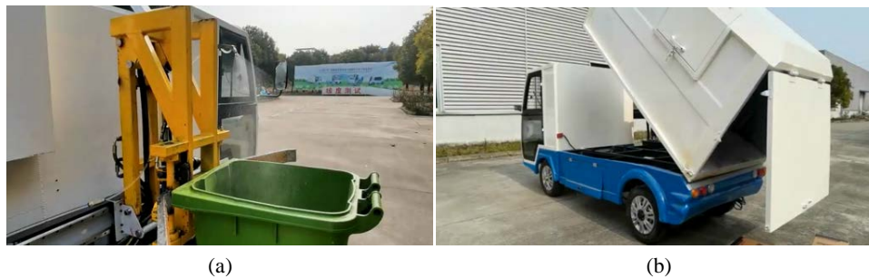
Figure 8. Disinfection and dumping of garbage bin: (a) disinfection, (b) overall dumping 图 8. 垃圾桶的消毒、倾卸动作: (a) 消毒, (b) 整体倾卸
