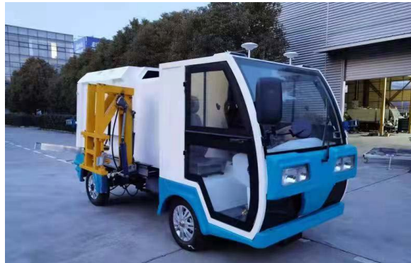
Figure 1. Automatic driving garbage recycling sanitation vehicle 图 1. 无人驾驶垃圾收集车
