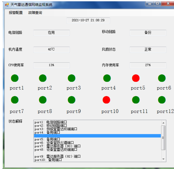
Figure 2. Main interface of monitoring system 图 2. 监视系统主界面
