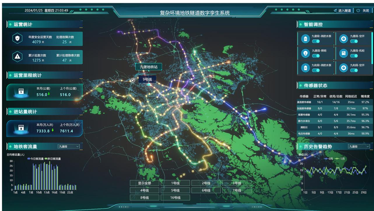
Figure 4. Main interface of digital twin system for subway tunnels
