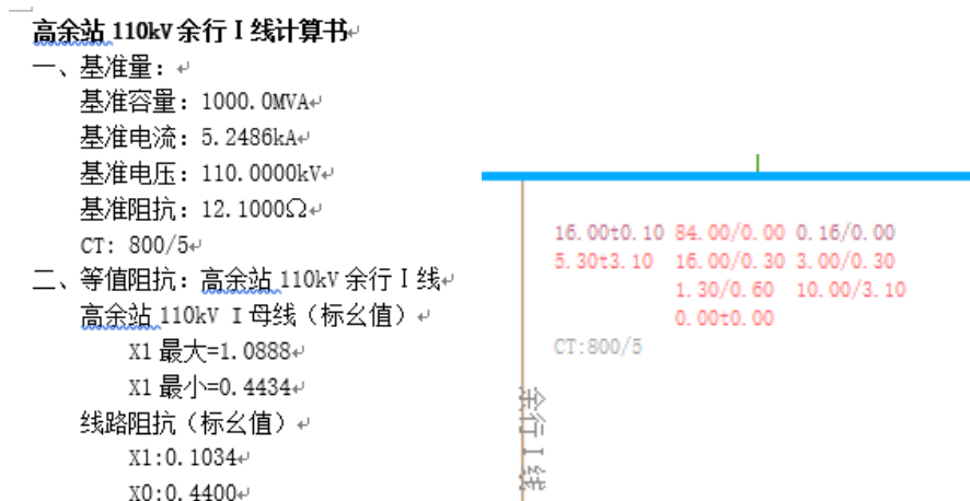
Figure 9. Automatic calculation of line protection setting
