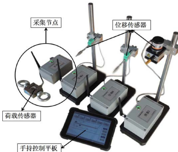
Figure 1. Wireless pole deflection measuring system
