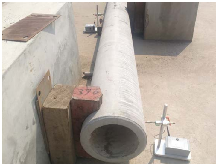
Figure 8. Field test of wireless pole deflection measurement system
