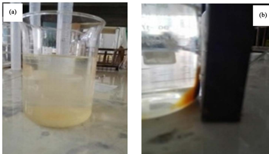
Figure 7. Produces yellow precipitate (a) at the end of the reaction and magnetic recovery (b) 图 7. 反应结束产生黄色沉淀(a)和磁力回收(b)
