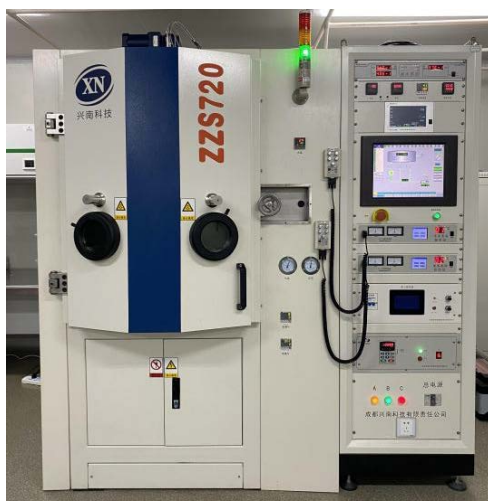
Figure 1. ZZS720 vacuum coating machine diagram 图 1. ZZS720 型真空镀膜机图
