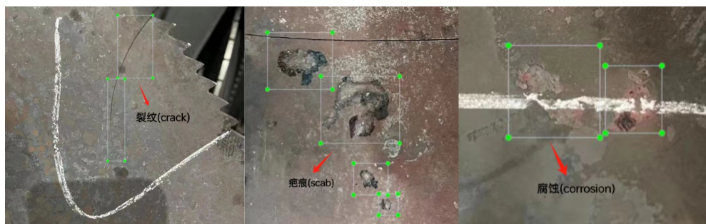
Figure 2. Saw blade defect annotation
