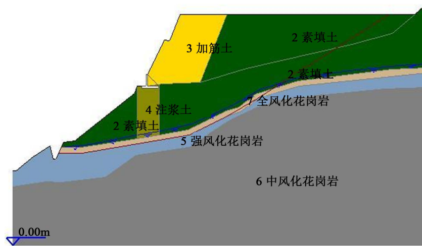
Figure 11. 3-3' section fold linear slide plane calculation model
