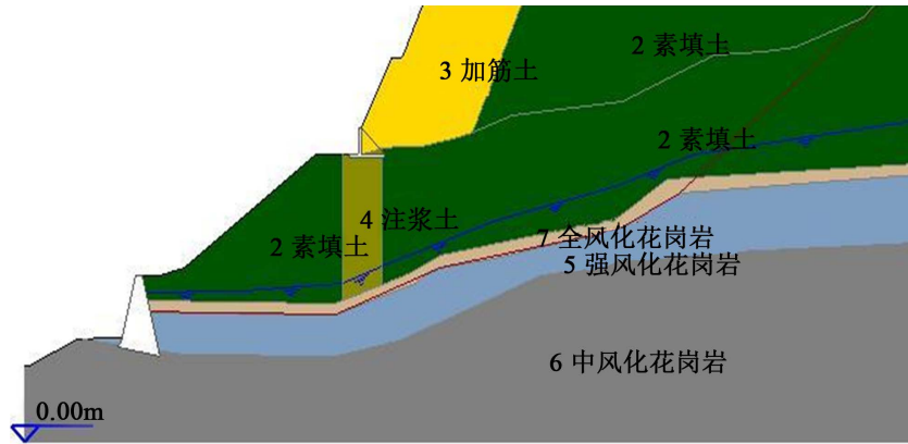
Figure 10. 2-2' section fold linear slide plane calculation model
