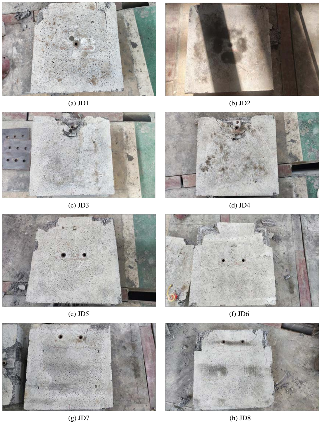
Figure 3. Failure mode of the specimens JD1~JD8 图 3. JD1~JD8 试件破坏形态
