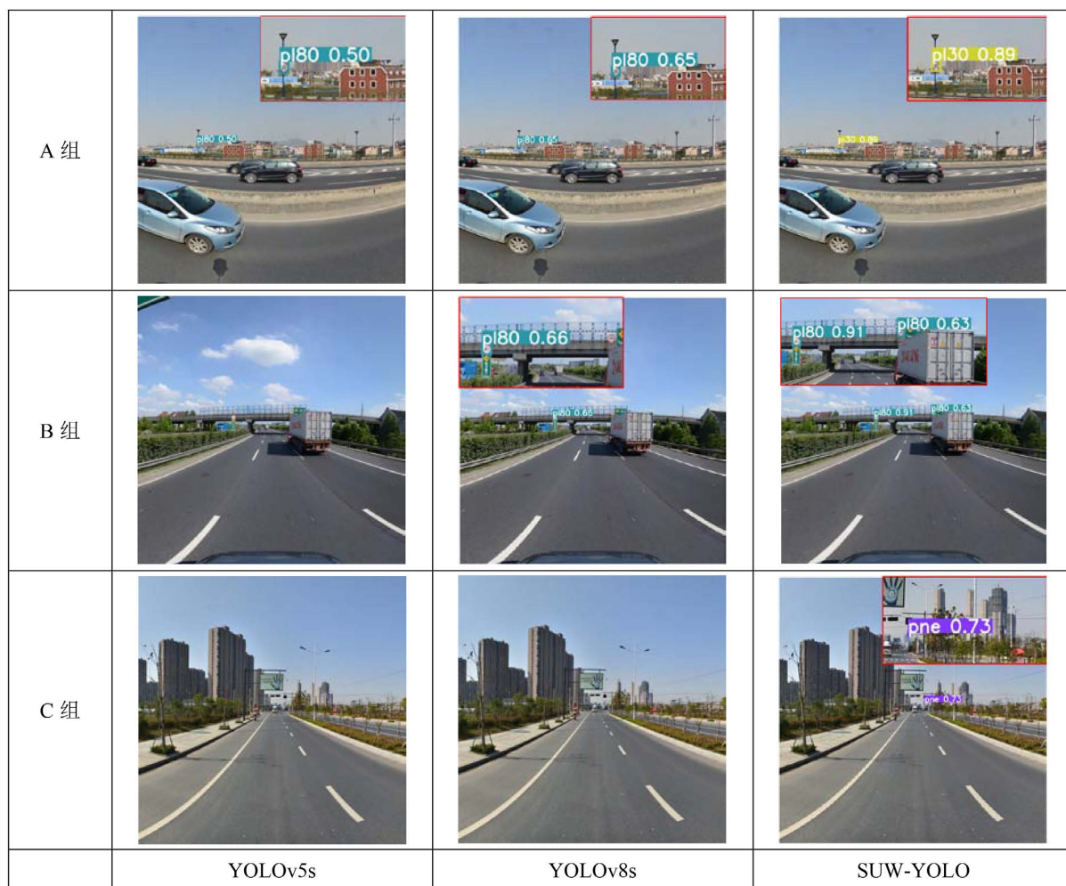
Figure 4. Comparison of traffic sign detection effect
