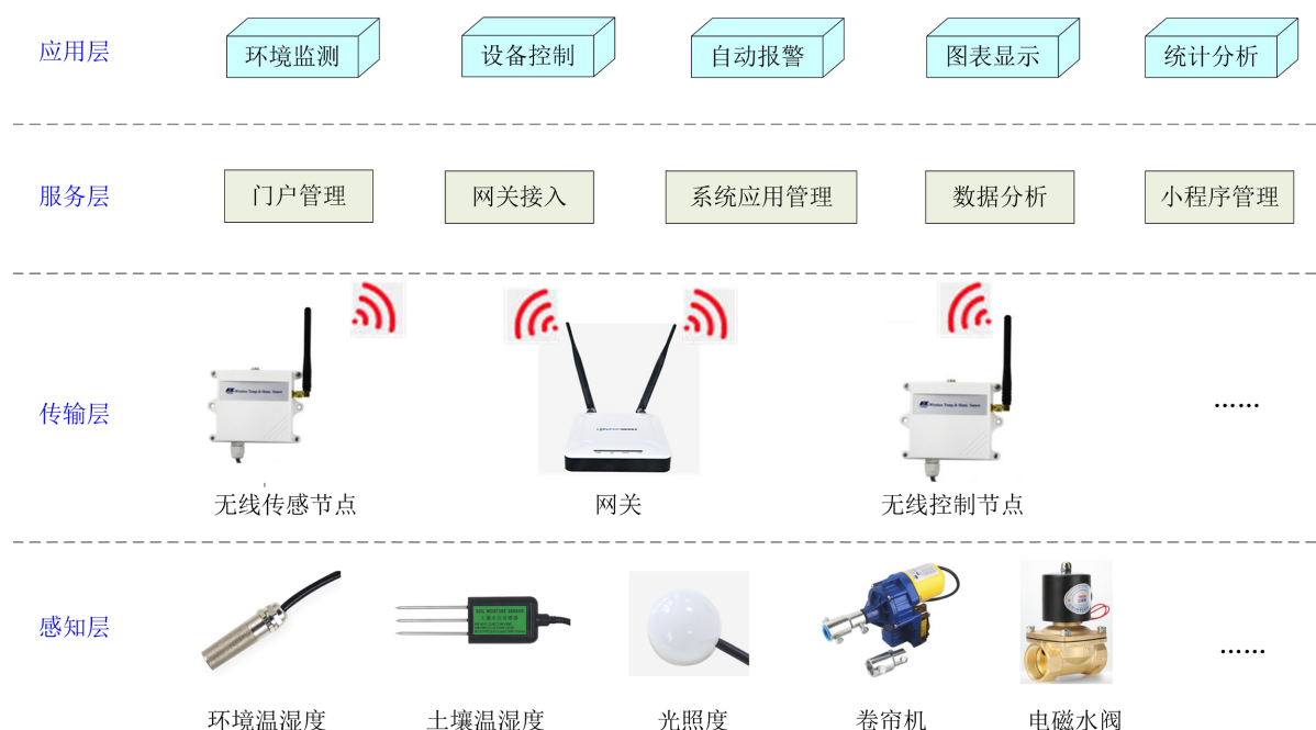
Figure 1. Diagram of layered architecture of the training platform system
