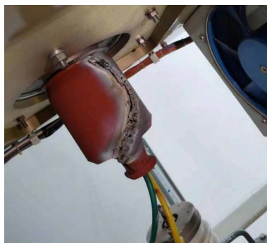
Figure 4. Breakdown diagram of cathode insulation of klystron
