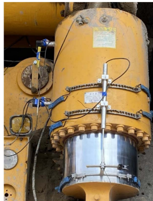
Figure 2. Installation of pressure and displacement sensors on rear suspension 图 2. 后悬压力和位移传感器的安装
