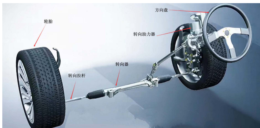
Figure 3. Mechanical structure of the autonomous steering wheel return system 图 3. 方向盘自主回正系统机械结构
