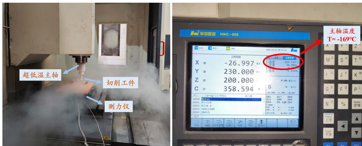
Figure 8. Liquid nitrogen assisted cooling cryogenic milling processing site 图 8. 液氮辅助冷却超低温铣削加工现场
