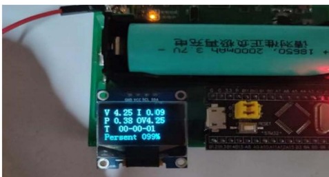
Figure 14. Check the battery for power on test
