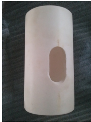
Figure 2. Structural diagram of ceramic nozzle 图 2. 陶瓷喷嘴结构图
