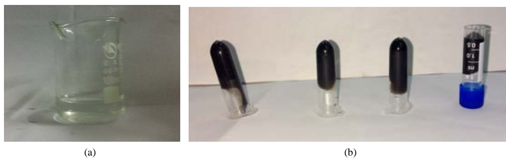
Figure 2. (a) Hyaluronic acid solution, (b) The macroscopic morphology of HA-DAP hydrogel 图 2. (a) 透明质酸溶液, (b) HA-DAP 水凝胶的宏观形貌图
