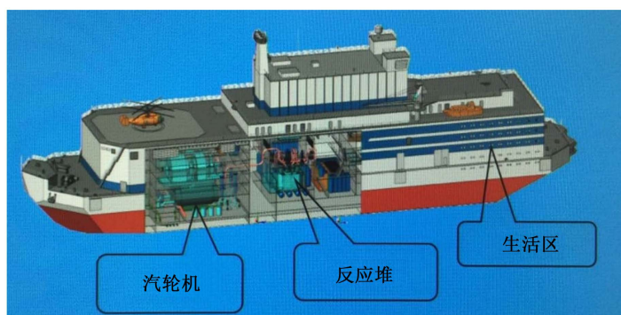
Figure 1. Typical structure of offshore floating nuclear power plant
