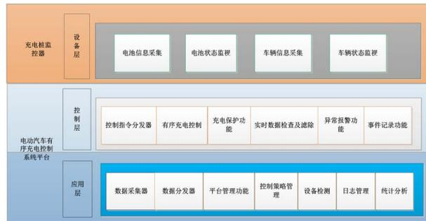
Figure 1. System framework of the charging pile centralized supervisory control
